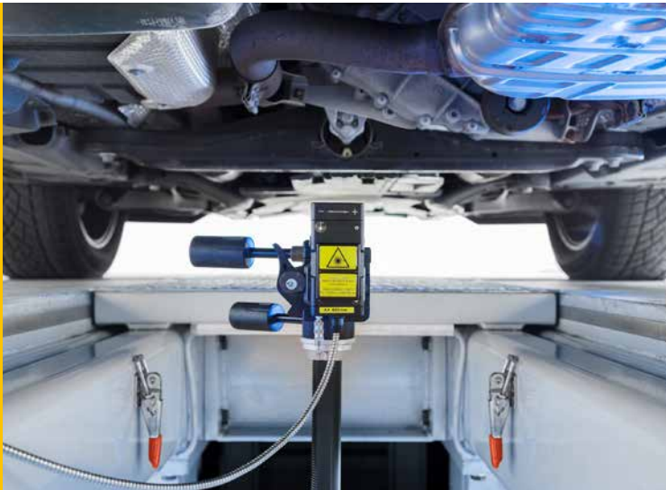
Torsional resonance assessment of a drive train on a rolling road. courtesy IPEK, KIT Karlsruhe, Germany
