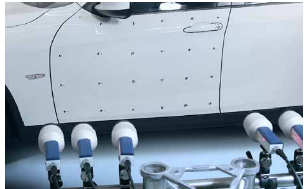
Synchronous optical vibrometry with a MPV Multipoint Vibrometer for acoustic analysis in door-slam tests or to study other transient or unstationary phenomena.
