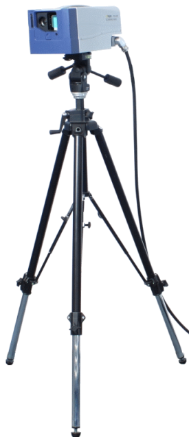
Figure 3.10: Scanning head mounted on the light duty tripod with fluid head
